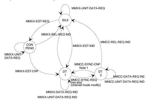
NOTE 1: the parameters in RR\_SYNC\_CNF must correspond to the parameter in RR\_SYNC\_REQ.
