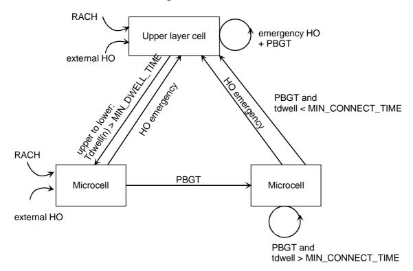
Figure C.3: Handovers in case of availability of the target cell
