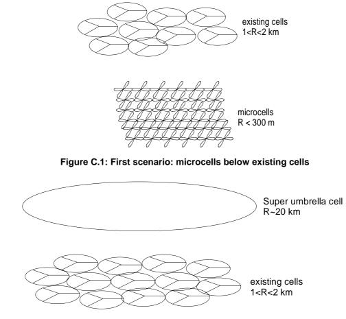
Figure C.2: Second scenario: "super umbrella cell" above existing minicells
