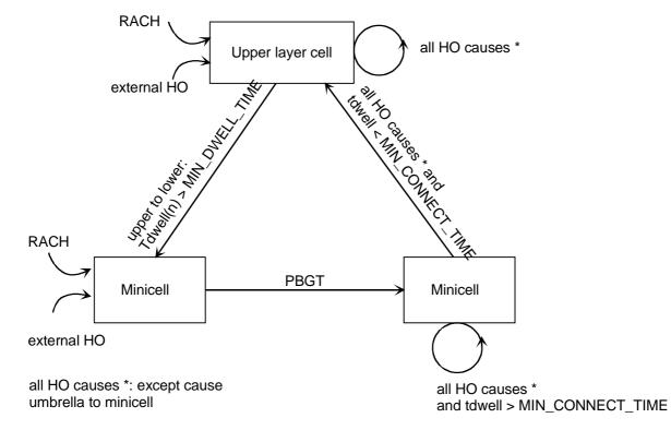
Figure C.6: Simplified handover diagram for minicells
