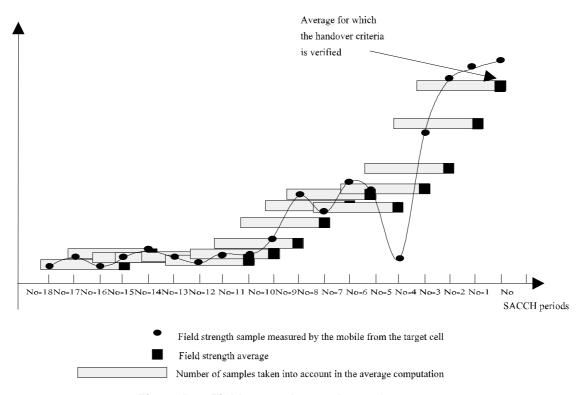
Figure D.2: Field strength samples and averages
