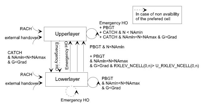
The handover that may occur to non preferred target cells due to the unavailability of TCH resources are indicated with dotted line arrows in the state diagram.
